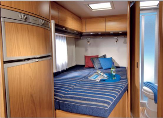
Restful sleep: Double bed with high-quality pocket-sprung mattress on a flexibly mounted slatted frame. Below that, a large storage compartment, accessible from inside and out.
