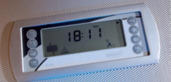
Service panel: Digital display of battery charge state, water levels and other functions.
