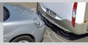
Manoeuvring aid: reverse driving sensors for reliable monitoring of the space behind the vehicle.
